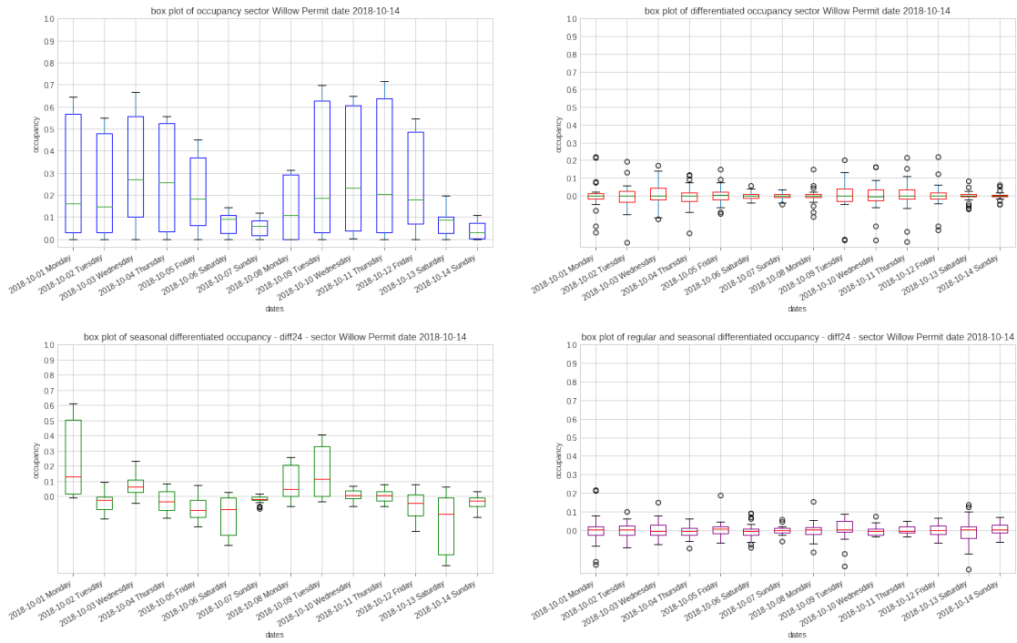
Figure 6.38: Daily box plots of the Los Angeles Permit sector from the first two weeks of October 2018 under different numbers of differentiations: no differentiation (top left), one regular differentiation (top right), one seasonal differentiation (bottom left) and one regular plus one seasonal differentiation (bottom right).
