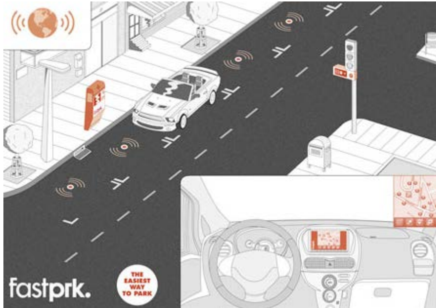
Figure 2.1: Physical components of the data pipeline. Once a node detects a change in their measurements (a car over it), the data is sent to a gateway (the component in the traffic light) that also sends the data to the cloud. Source https://www.worldsensing.com/product/fastprk/
