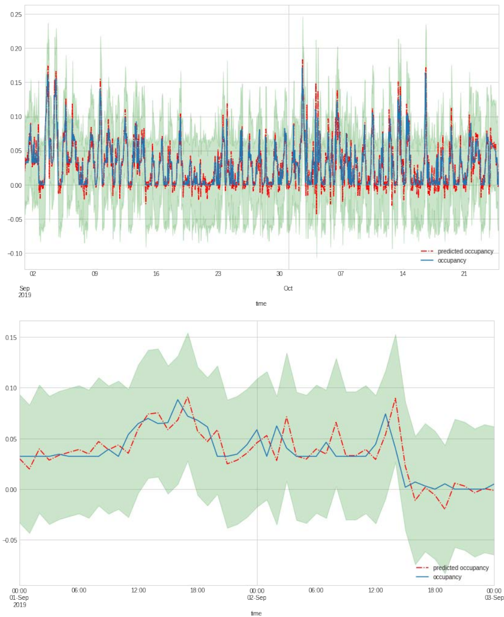
Figure 6.42: ARIMA forecasts from the proposed model for sector Permit from Los Angeles. Left presents forecasts for all the out-of-sample interval while right the first two days of the same interval of time. Blue denotes the observed occupancy, red the forecasted by the model and green is the confidence interval.
