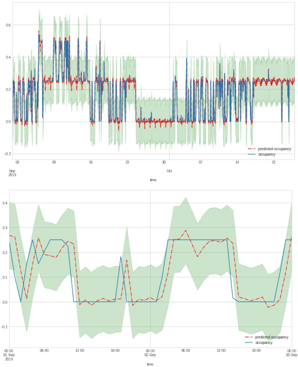
Figure 6.52: ARIMA forecasts from the model proposed for the ZipCar sector in Los Angeles. Top presents forecasts for the entire out-of-sample interval while bottom is the first two days of the same interval of time. Blue denotes the observed occupancy, red the occupancy forecasted by the model and green is the confidence interval.
