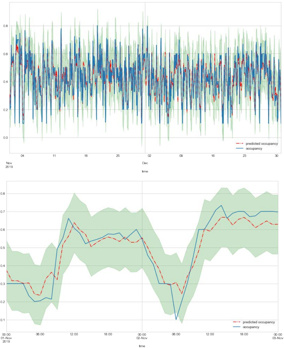
Figure 6.10: Antwerp Van Wesenbekestraat Zone 1 ARIMA forecasts. Blue denotes the observed occupancy, red the occupancy forecasted by the model and green is the confidence interval. Top presents the entire out-of-sample interval of data while bottom presents out-of-sample predictions for two days.
