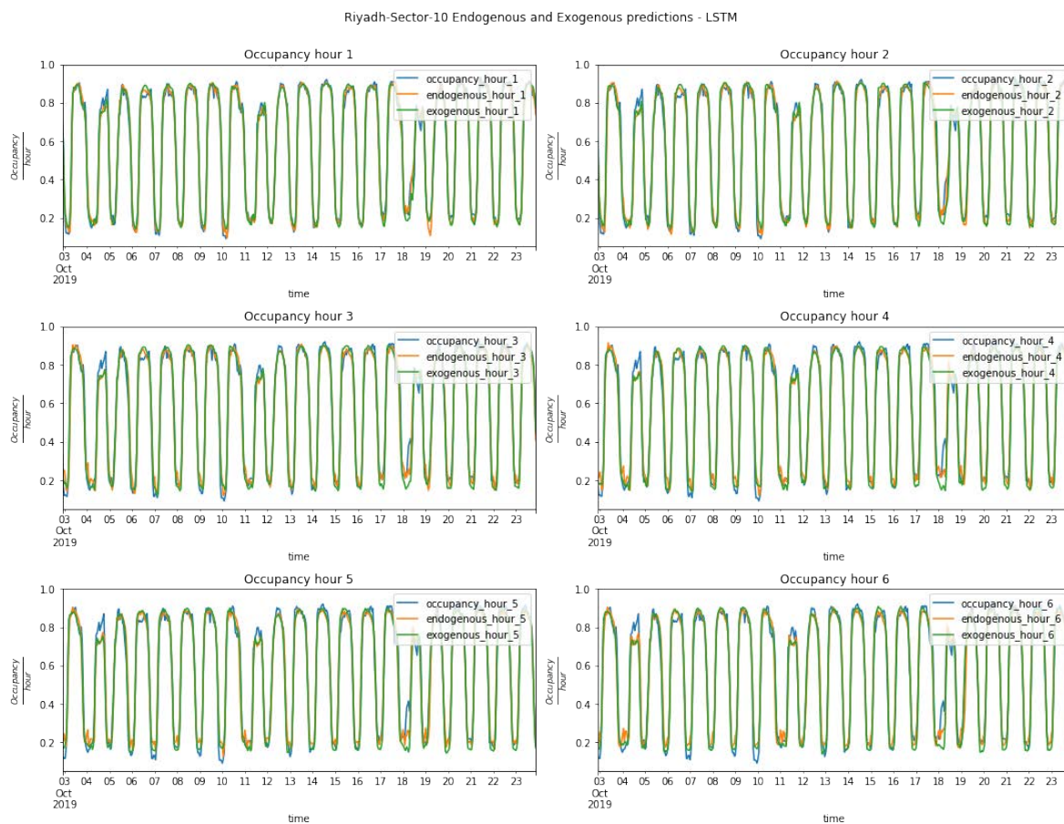
Figure 9.13: Riyadh Sector-10 LSTM model forecasts comparison. Blue belongs to the true parking occupancy, orange to the forecasts from the endogenous model and green to the forecasts from the exogenous model.
