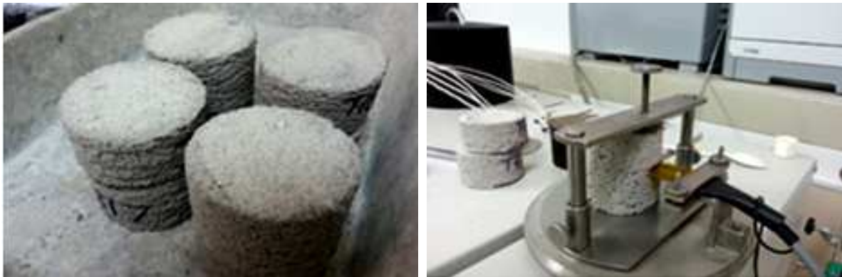
Figure 1, The samples and experimental setup of Hot Disk Thermal Constant Analyzer test
