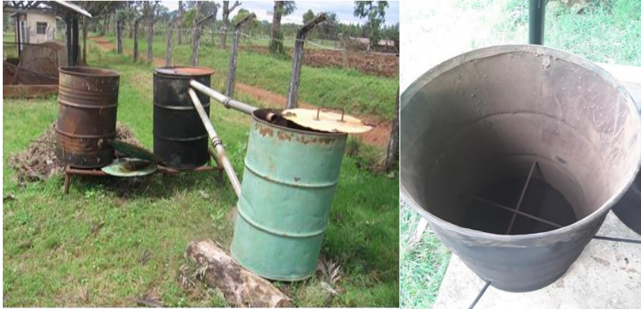
Drums for steam sterilisation of substrate
