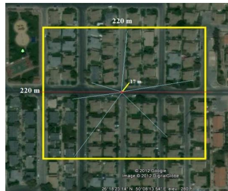
Figure 5. 64-buildings in Al-Dhahran with Single BS located at the centre of the scenario
