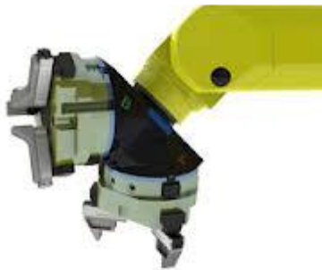
Figure 3: End effector with double grippers
