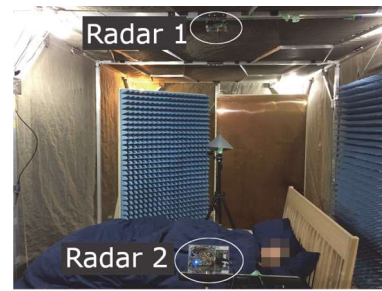
Fig. 3 Measurement setup with a pair of radar systems and a participant lying in a bed.
