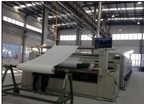
Fig. 2. Heat setting is carried out with stenter machine.
