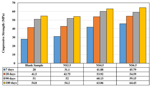
Fig. 1. Compressive strength of samples at various ages: 7, 28, 90, and 180 days [34].
