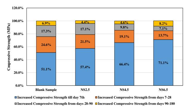
Fig. 2. Acquired compressive strength at 7, 28, and 90 days in comparison to strength at 180 days.
