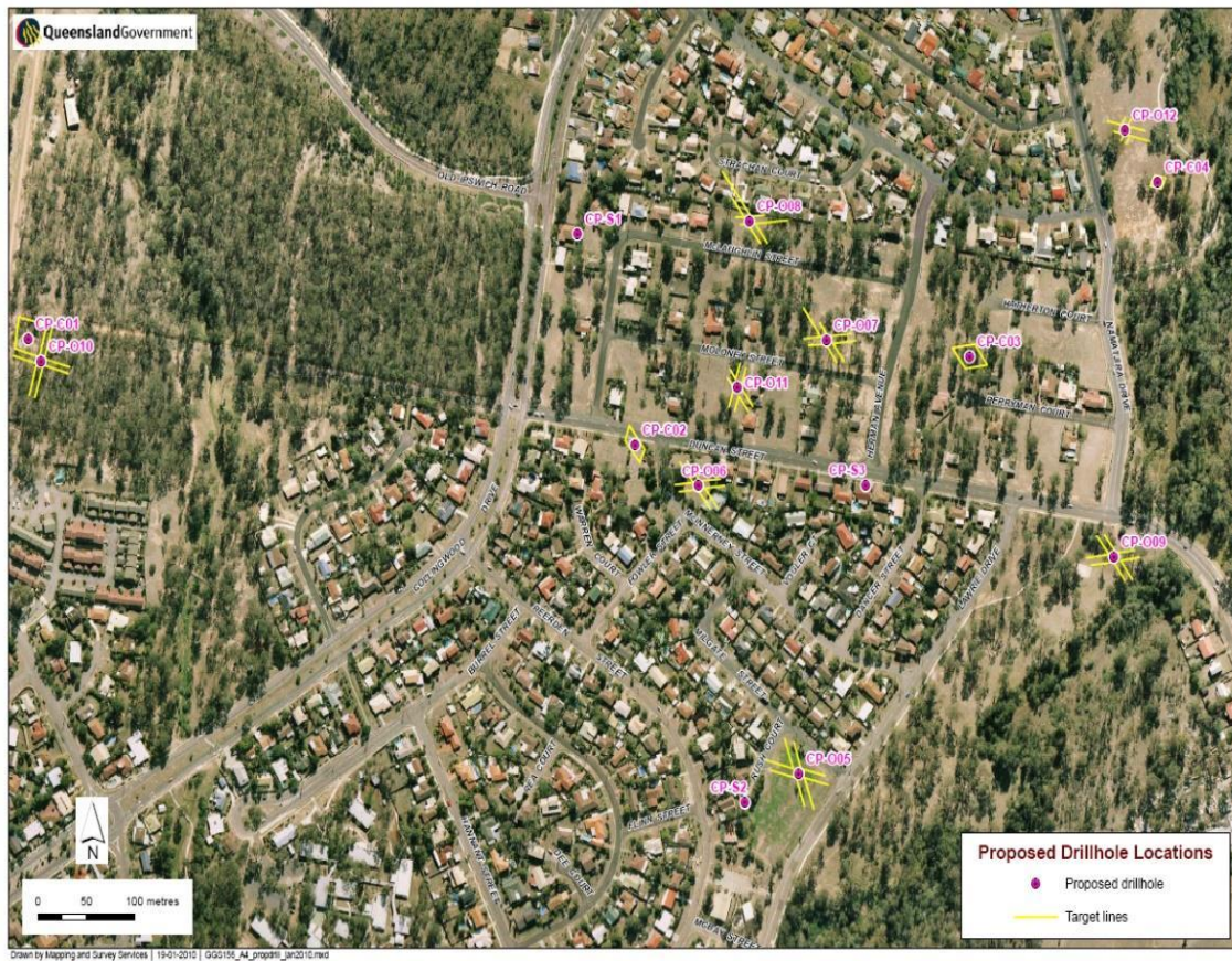
Figure 1: Locations of 15 drill holes designed by CSIRO distributed in both historical subsided and non-subsided areas (Shen et al, 2010)
