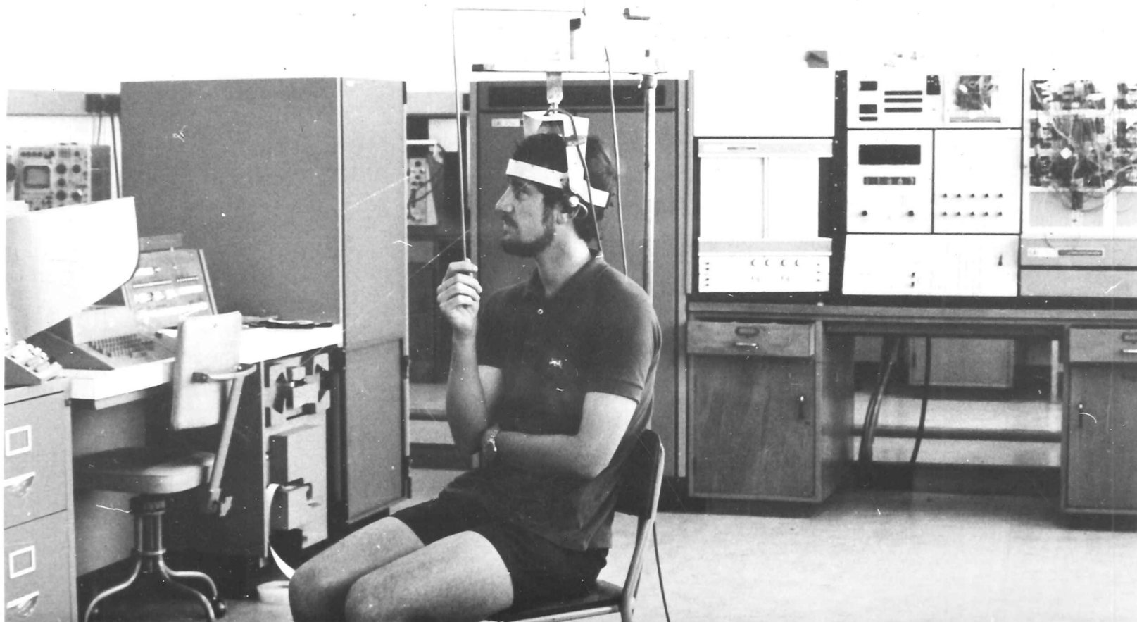
Plate 8.1 Equipment and computing facilities used in the interactive localization experiments. The subject's head position is monitored by the sliding vane attached to his headset and the image direction indicator is affixed to the boom above the head. (The EAI 640 digital computer is to the left, the EAI 693 hybrid linkage unit is behind the subject, and the EAI 580 analogue computer is at right).
