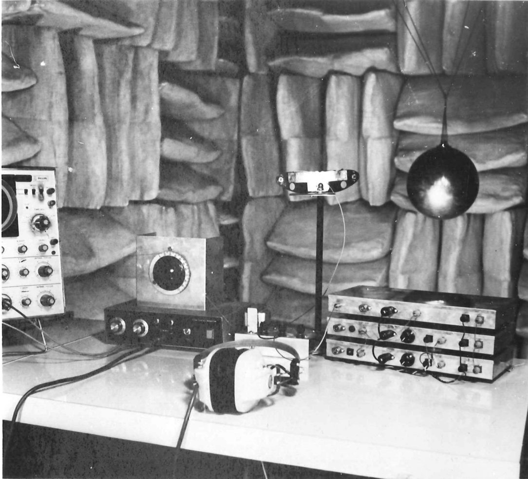
Plate 3.1 The prototype binaural echolocation system in the experimental environment for localization experiments.
