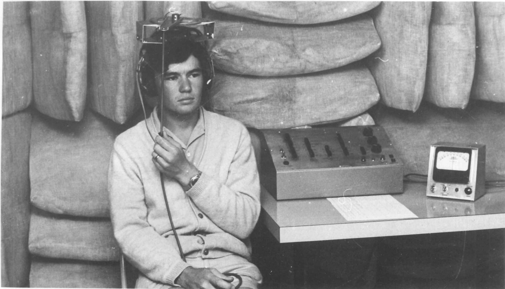
Plate 4.1 Equipment used in dichotic IAD localization experiment. The subject is holding the image direction indicator; the meter at right provides a remote readout.
