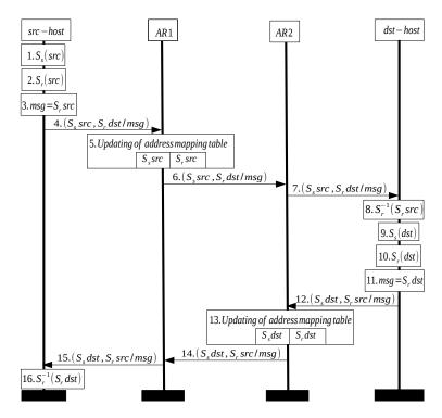
Figure 5.3: uOTA Routing Packets.
