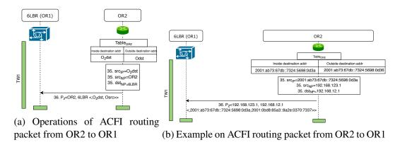
Figure 6.13: ACFI routing packet from OR2 to OR1 (6LBR)
