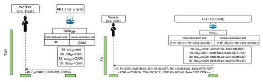
(a) Operations of ACFI routing (b) Example on ACFI routing packet from AR1 to Source packet from AR1 to Source Host
