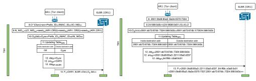
(a) Operations of the communication (b) Example on the communication between between AR1 and 6LBR AR1 and 6LBR
