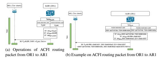
Figure 6.14: ACFI routing packet from OR1 to AR1
