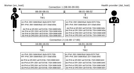
Figure 6.16: Results of ACFI communication between worker and health provider in two different connections
