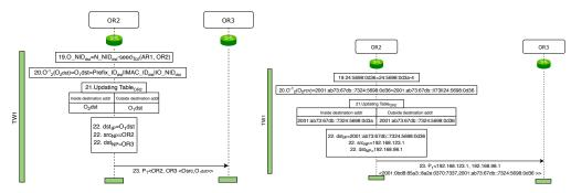
(a) Operations of the communication (b) Example on the communication between between OR2 and OR3
