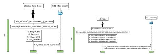
(a) Operations of the communica- (b) Example on the communication between tion between Source Host and AR1 Source Host and AR1
