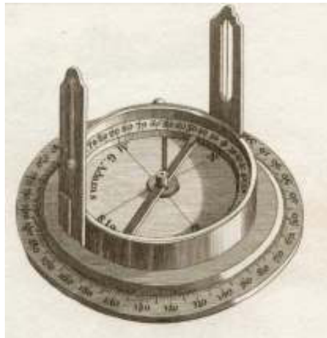
Figure 4.11 The ‘plain’ theodolite (circumferentor) used on the ‘Military Survey of Scotland’ 407
