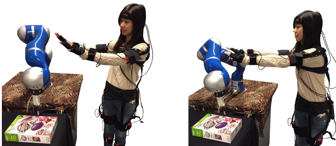
Figure 9.1: Robot-human close interaction. Left figure shows the robot's original motion, the right figure shows the adapted motion when human subject pushes her hands to block the original trajectory.
