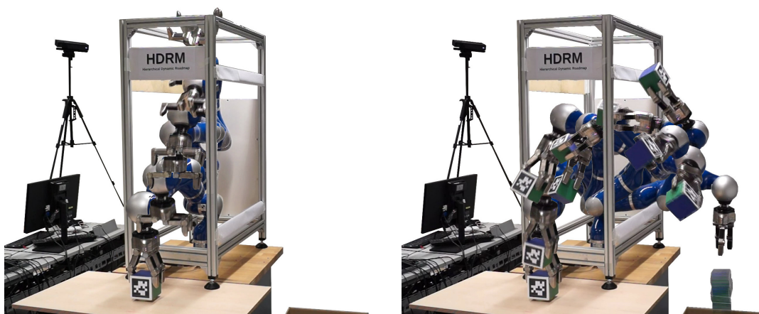
Figure 6.1: The 7-DoF KUKA LWR robot with Dexterous Hand operating inside a cage. Left: grasping the target from upright posture; right: dropping the object to the side.
