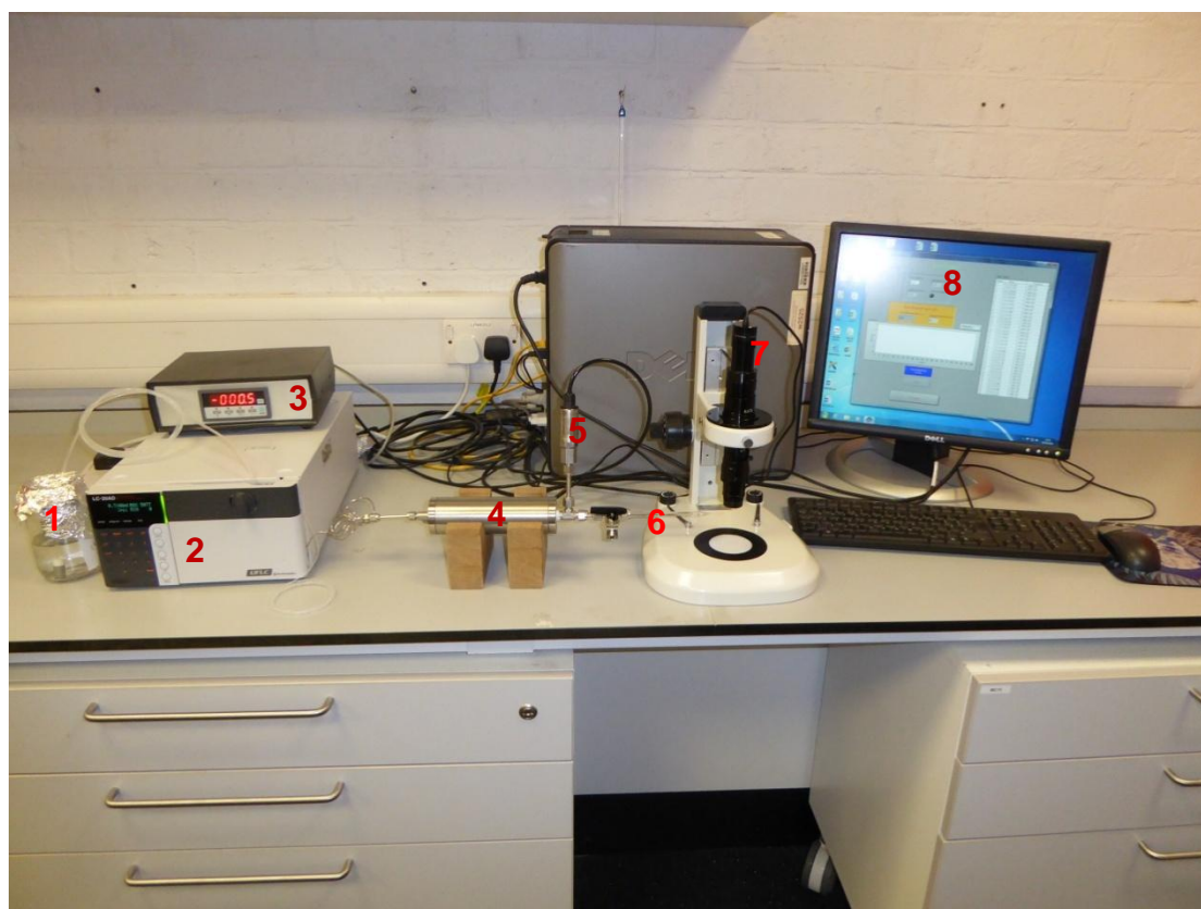
Figure 3.1: Experimental setup for measurement of resistance to flow path in a capillary: (1) water reservoir (2) pump, (3) digital pressure display, (4) stainless steel cylinder, (5) transducer, (6) glass tube with tapered capillary at the end under a travelling microscope, (7) digital camera, (8) computer with LabView.
