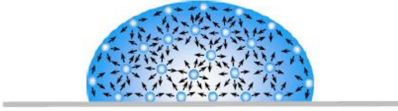
Figure 2.21: Unbalanced forces of liquid molecules at the surface causing surface tension (Yuan and Lee, 2013).
