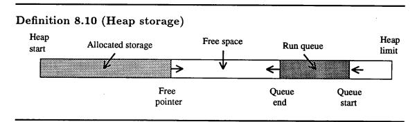
As we add entries to the end of the run queue, it grows towards the middle of the heap. Similarly, as we allocate memory in the ordinary part of the heap, the free pointer moves towards the centre of the heap. This memory model has the benefit that we need only perform a single test to determine whether we need to do a garbage collection (we just test whether the difference between the end of the run queue and the free pointer is sufficiently large for the allocation we wish to do).
