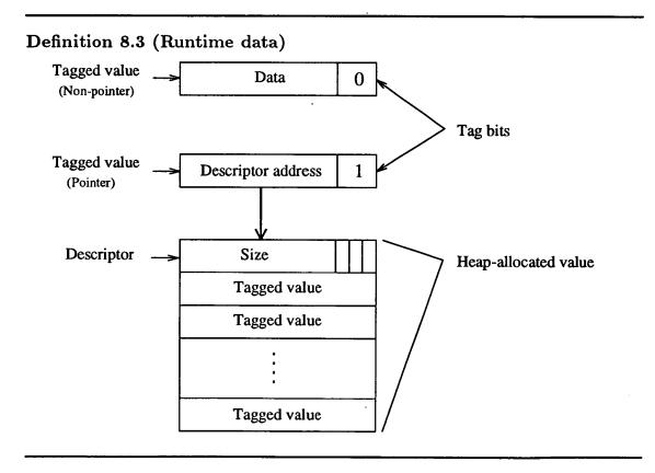
The above picture describes the general format of our runtime data. A zero tag bit indicates that a value is not a pointer into the heap. A tag bit of one signifies that a value is a pointer to a heap-allocated object. Subtracting one from such a value yields the address of a *descriptor* in the heap, which gives further details about the type of the object.
