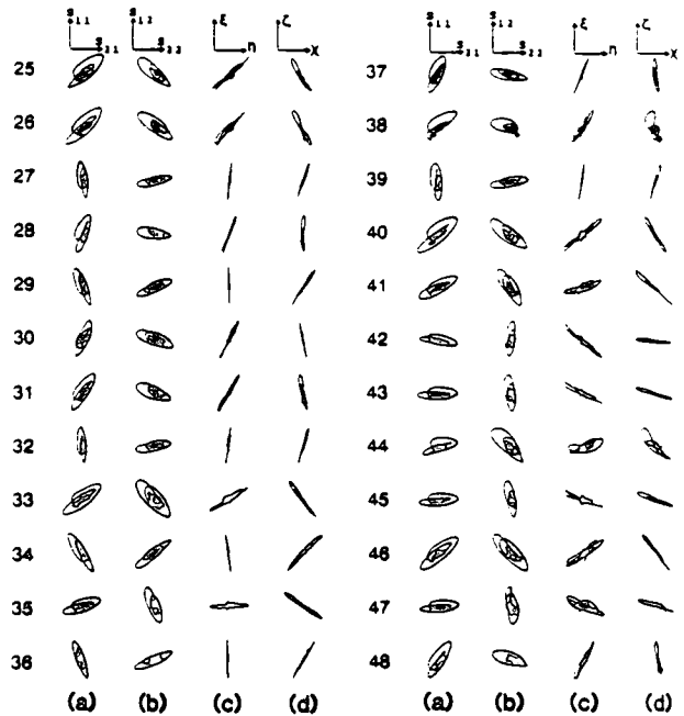
FIG. 2. Polarization diagrams (PDs) of a zero-offset VSP from BP, showing the linearity of the transformed motions: (a) in-line source ( X -source), s_{11}(t) and s_{21}(t) ; (b) cross-line source ( Y -source), s_{12}(t) and s_{22}(t) ; (c) transformed components, \xi(t) = s_{11}(t) - s_{22}(t) and \eta(t) = s_{12}(t) + s_{21}(t) ; and (d) transformed components \zeta(t) = s_{11}(t) + s_{22}(t) and \chi(t) = s_{12}(t) - s_{21}(t) .
