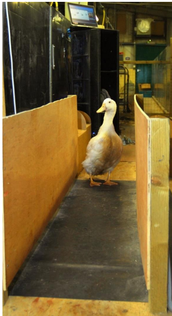
Fig. 2. A Pekin duck ready to walk over a pressure walkway (which is hidden under latex sheeting to provide the bird with grip). Data is recorded on the laptop in the background.
