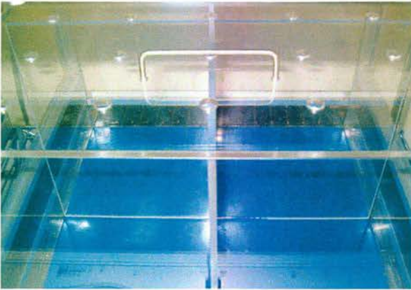
Figure 2.1 Activity monitor chambers (top) and an individual mouse activity arenas (bottom). Animals are placed in each chamber and all movements are recorded via infrared beam breaks.
