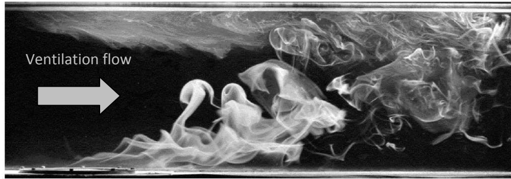
Figure 7: Photograph of a small scale tunnel fire during the occurrence of back-layering. The fire size is 15 kW. The tunnel has an arched cross section (width 274mm, height 244 mm). Adapted from [33].
