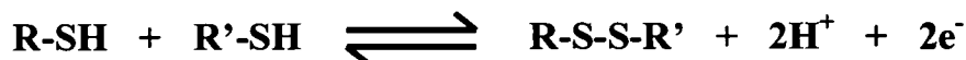
Fig 5.5: The general redox scheme describes the overall reactions that create (oxidize) or destroy (reduce) disulfide bonds
