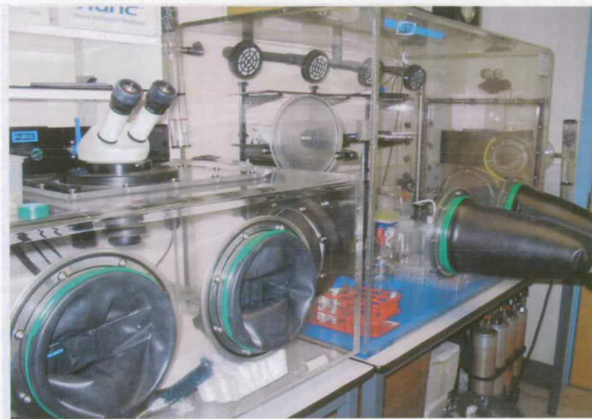
Fig 3.10: Belle technology anaerobic glove box. One side of the anaerobic box is adapted for the setting up of the crystallization experiments, while the other is fitted with a microscope for the observation and the manipulation of crystals
