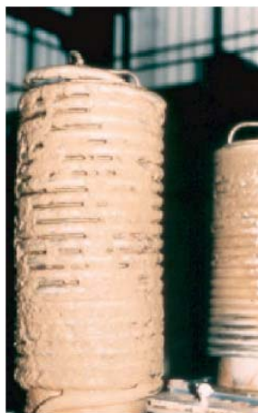
Figure 1.3 Biofouling of heat exchangers in process industry – from (Flemming, 2002)
