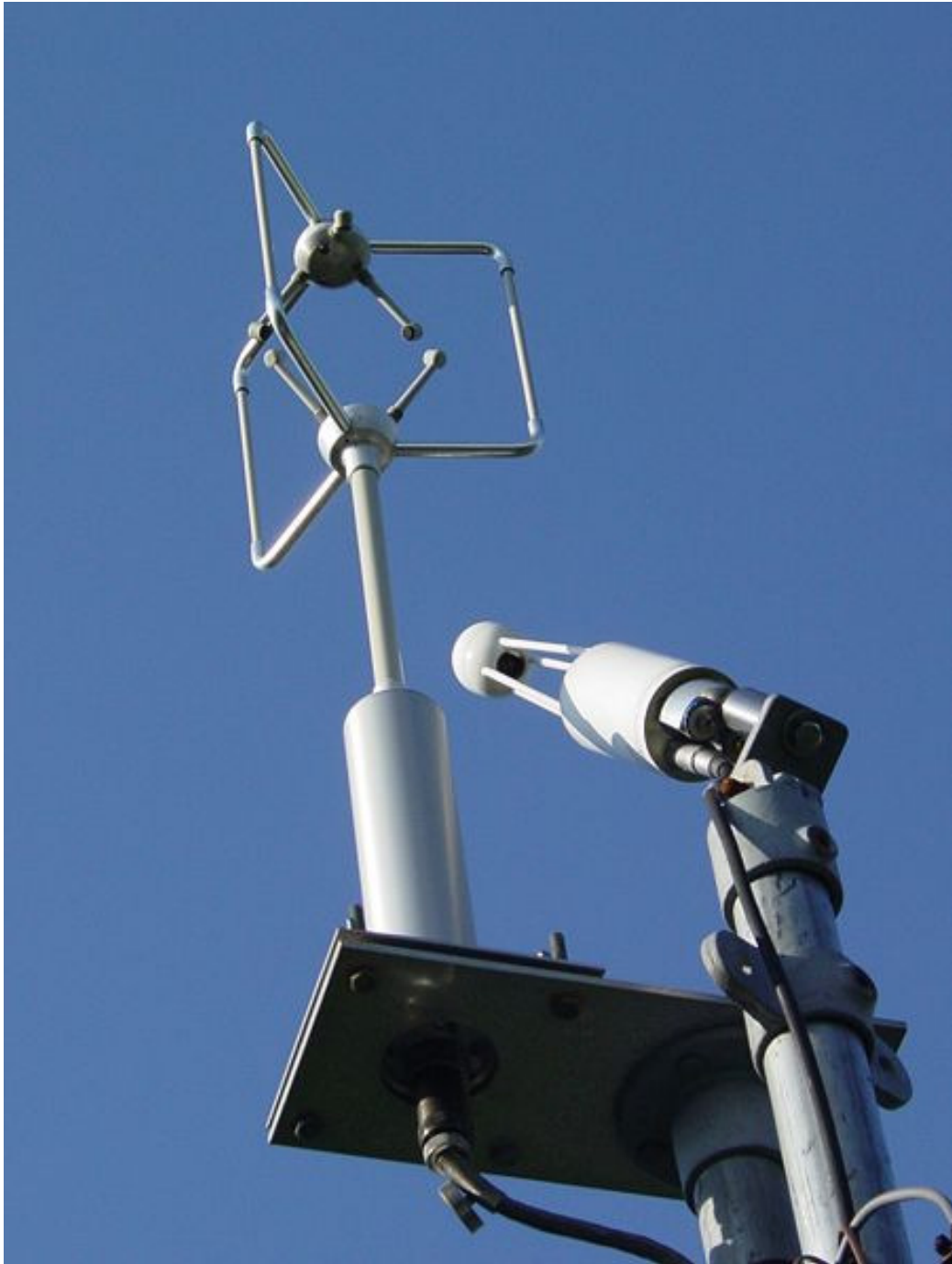
Figure 1-1 Eddy covariance sensor, consisting of a 3-axis ultrasonic anemometer and open path infrared gas analyser (IRGA), capable of measuring turbulent fluxes of carbon dioxide, latent heat, sensible heat and momentum. Photo courtesy of S.Dengel.
