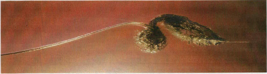
Figure 2.5: A surface roller and plunger vortex are forming after the splash at the plunge point. Photograph courtesy of Peter Tuffy and David Skyner.
