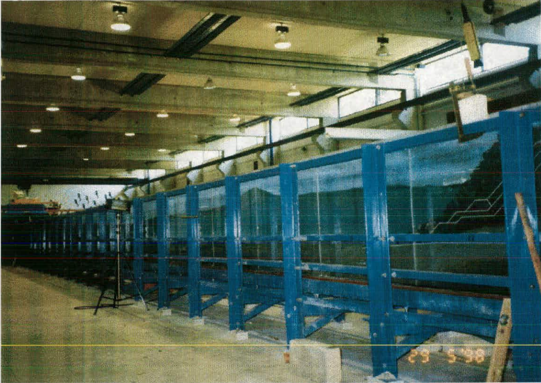
Figure 4.3: A photograph of the ISVA wave flume. A piston-type wavemaker is located at the far end (on the left hand side of the picture, unseen).
