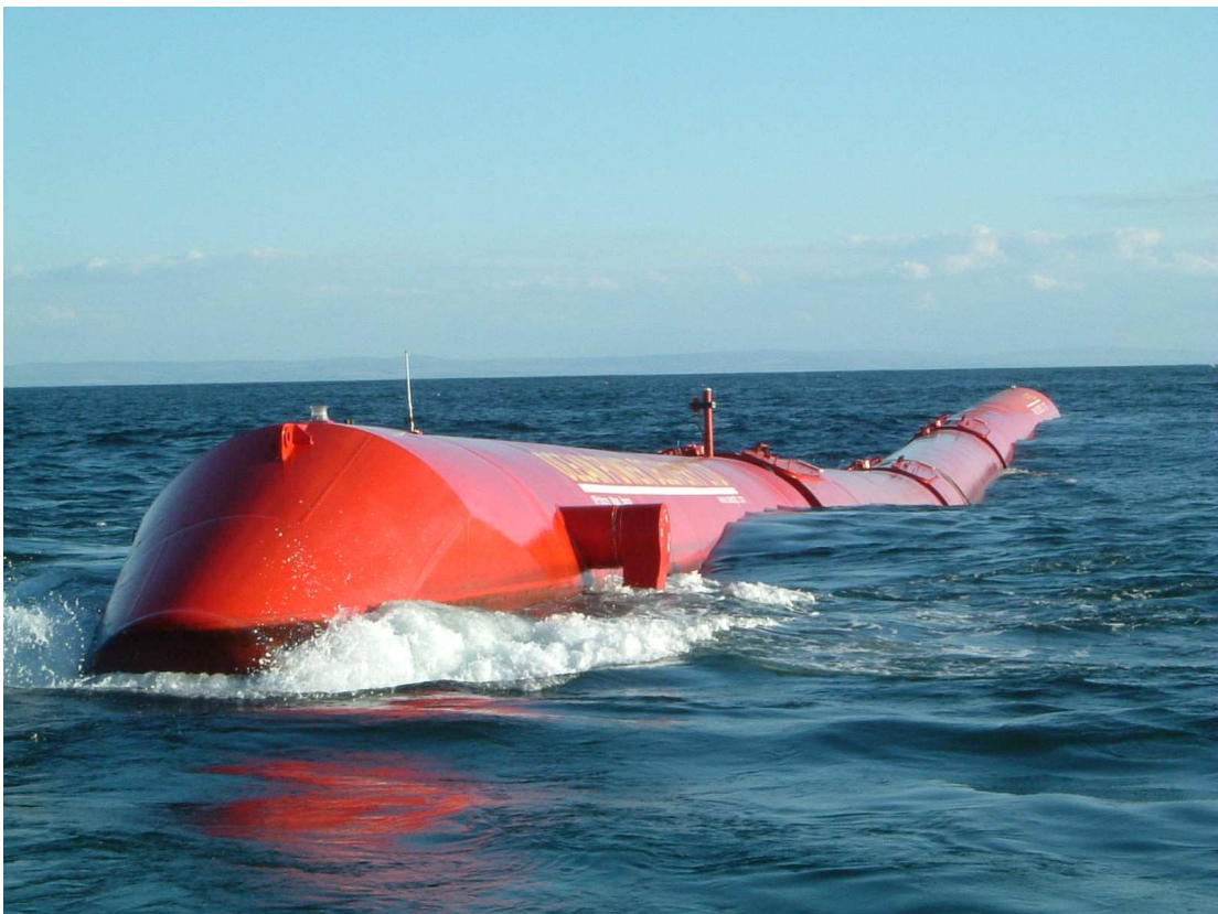
Figure 2.7: The Pelamis WEC: The P1 prototype undergoing sea trials.
