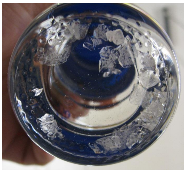
Figure 3-1 - Crystals of fumaric acid formed upon heating an aqueous maleic acid solution. Fumaric acid has much lower solubility which means the crystals form at high temperatures even when maleic acid is undersaturated. Bottle diameter 100 mm.
