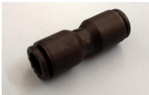
Figure 5-13 - Black plastic union which connects two 3 mm ID glass pipes together while maintaining consistent ID. This showed good alignment, but it was not possible to monitor formation of crystals at the joint.
