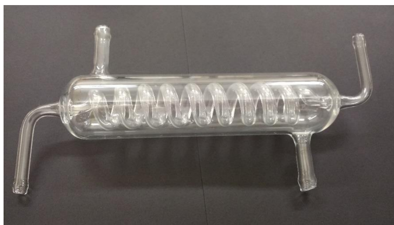
Figure 5-7 - Custom-manufactured cooling coil to fit 4.5 mm ID glass pipe. The internal coil with fused pipe (left to right) is surrounded by a water jacket with inlet/outlet top and bottom.
