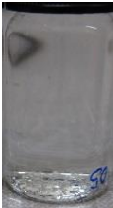
Figure 3-4 - Image of sulfamerazine crystals in acetonitrile fully matured to their maximum size. These crystals could not be detected for 2 days after growth, and even at maximum size were hard to detect by eye. For this example, S_{20} = 2 , giving 0.7 g excess SMZ per 120 g MeCN; per vial pictured is ~7 mg crystals formed. Vial width is 12 mm.
