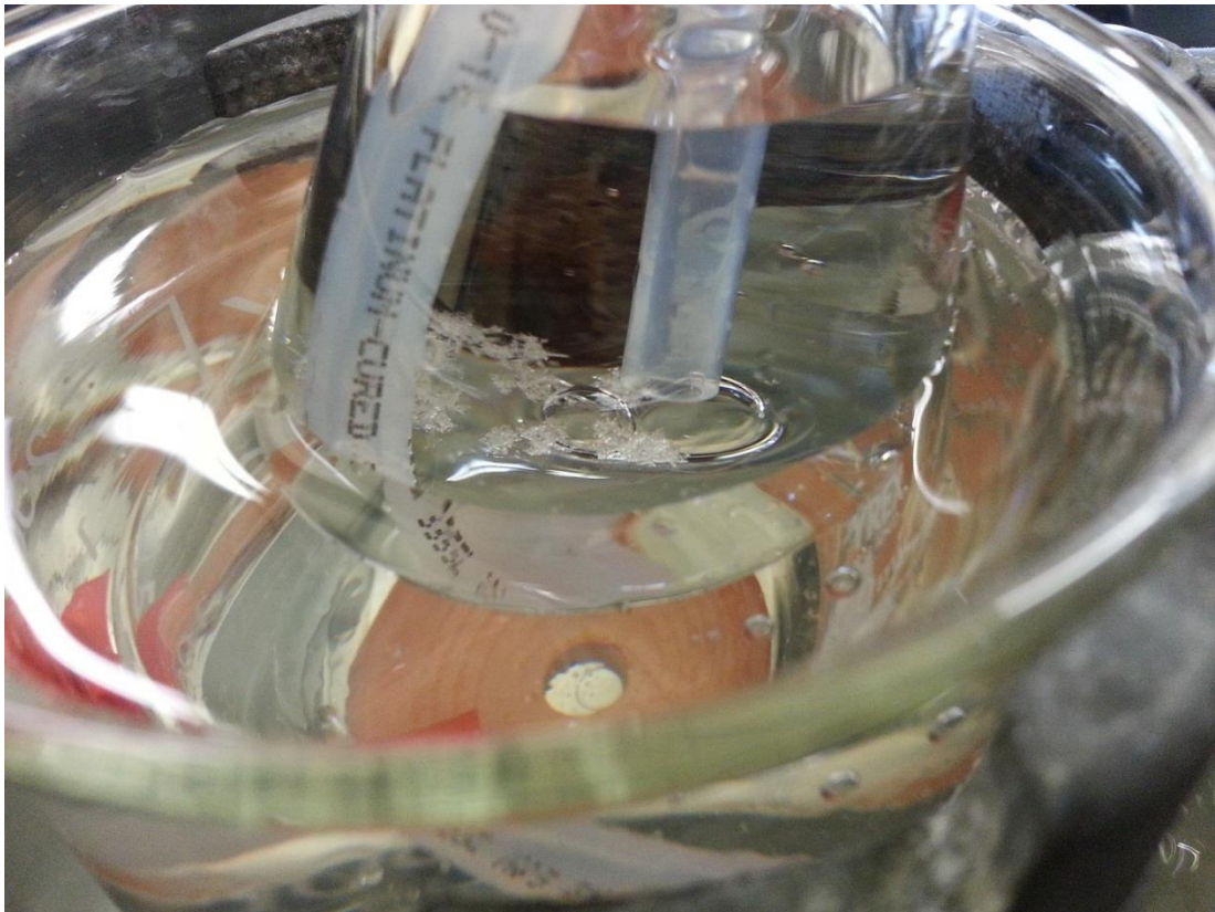
Figure 5-18 - Image of separator in beaker of water showing the two fluids (PFPE and aqueous ammonium chloride) forming an interface in the middle of the conical flask. At this interface sits crystals which had not dissolved in the tubing loop before entering the separator. This is undesired as it will lead to a concentration gradient in the aqueous layer.
