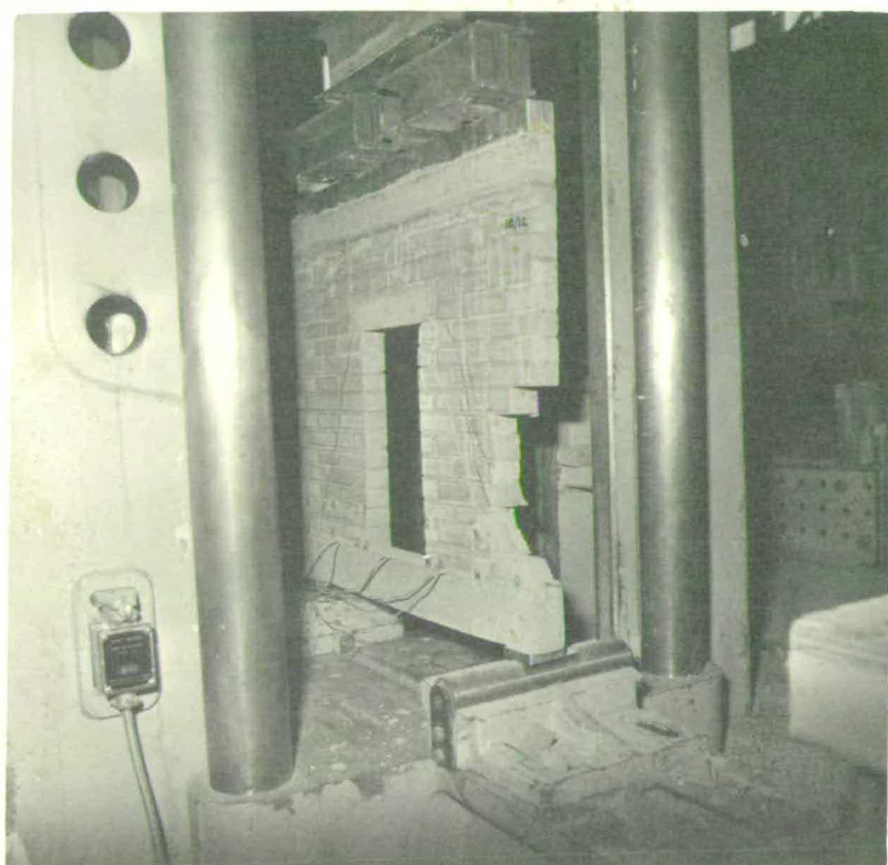
PLATE 8.1 WALL 10c AFTER FAILURE
