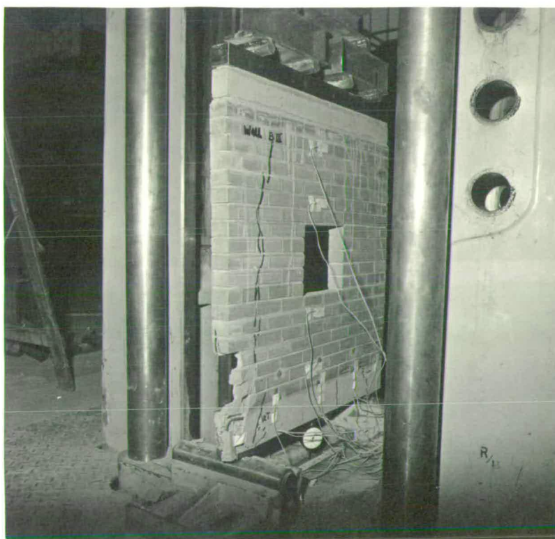
PLATE 6.2 WALL BIII AT FAILURE
