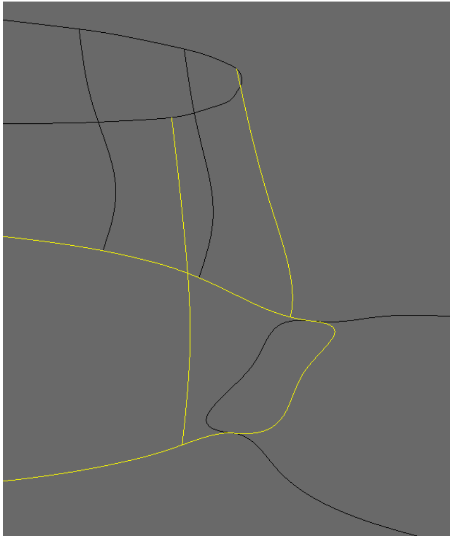
Figure D.10: Creating the upper curve that creates the start of the bifurcation outline at the top of the CCA.
