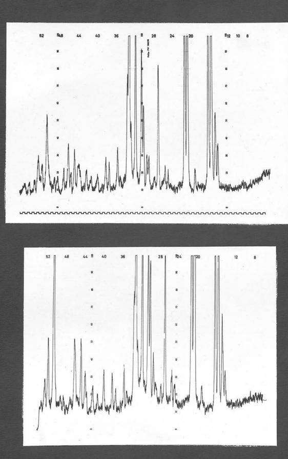
Fig. 31a X-ray Diffraction Pattern of a Mixed Whewellite
