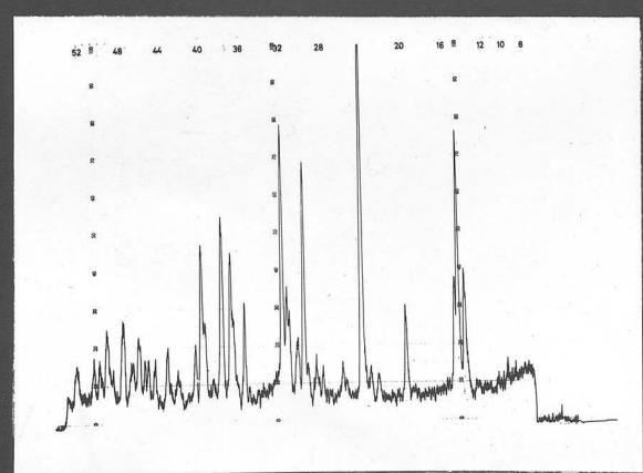
Fig. 32. X-ray Diffraction Pattern of a Weddellite Stone.
