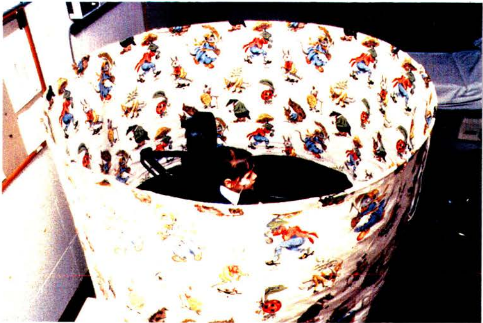
Large Drum used for Optokinetic Testing.
