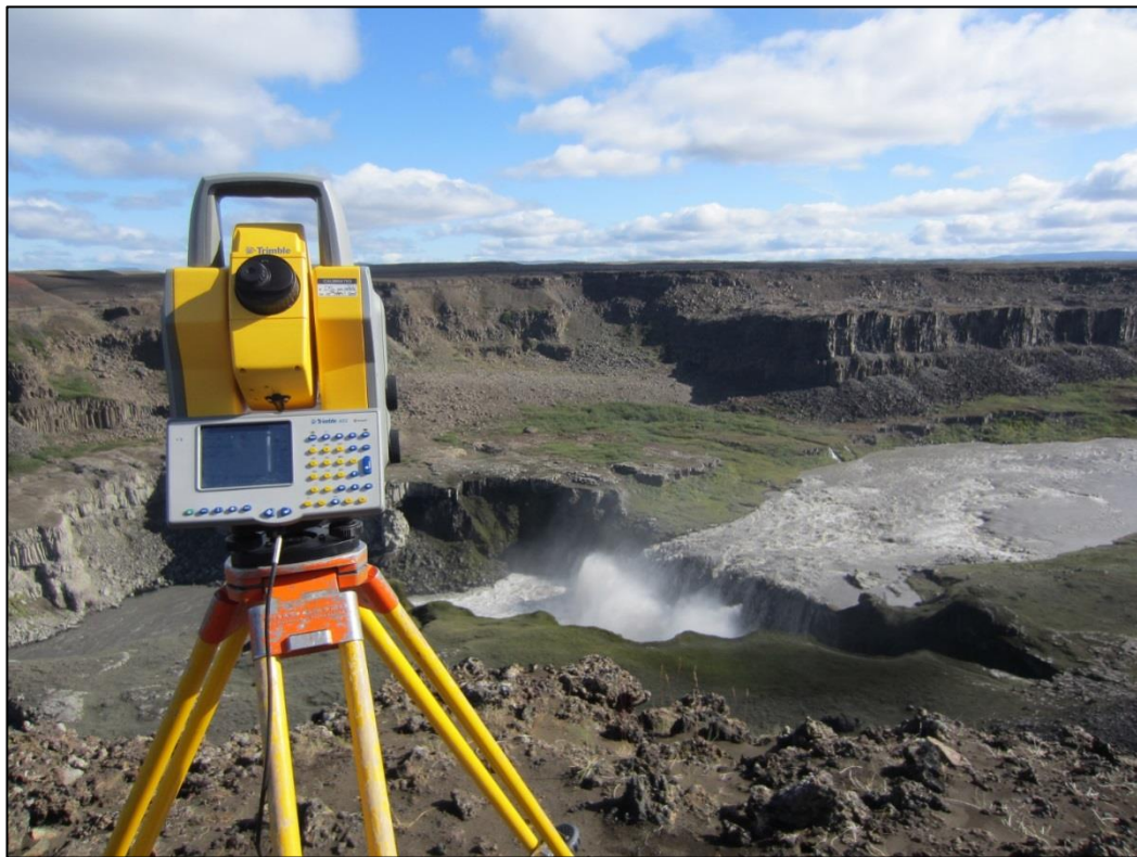
Fig. 2.2.4: Total Station survey location above Hafragilsfoss waterfall on the western wall of the Jökulsárgljúfur canyon. The Total Station surveys were carried out to provide highly accurate estimates of the heights and locations of strath terrace surfaces within the canyon. Photo taken looking east; for scale, Hafragilsfoss is 25 m in height.
