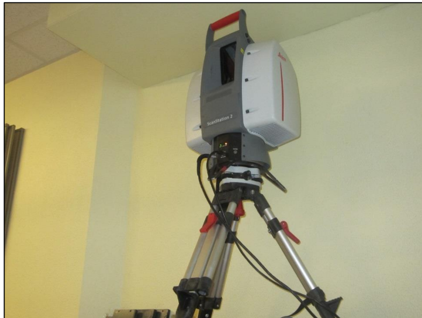
Fig. 3.2.1: The Leica ScanStation 2 Terrestrial Laser Scanner system used to collect the high resolution topographic data of the experimental channel every 60 seconds.
