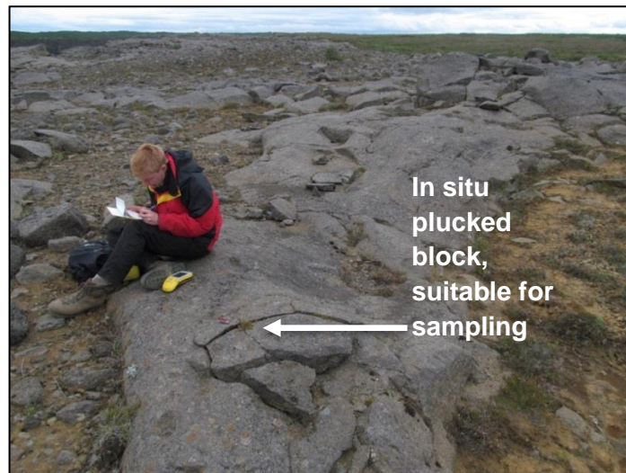
Fig. 2.2.13: Photograph showing an example of an in situ plucked block that has clearly not been transported far since detachment from the bedrock surface. Such a block is suitable for sampling. Sample: AI2 (Fig. 2.2.12)
