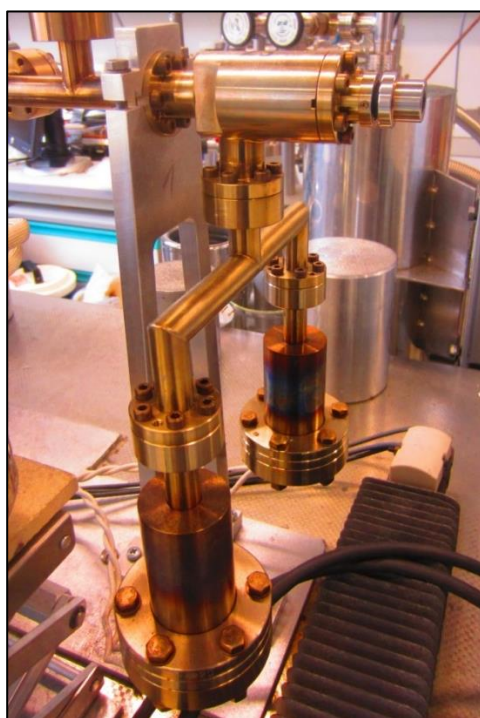
Fig. 2.2.22: The two SEAS (ZrAl) getters used to purify the gas before analysis. They absorb all the remaining active gases from within the vacuum, leaving the noble gases Argon, Krypton, Xenon, Helium and Neon for analysis.
