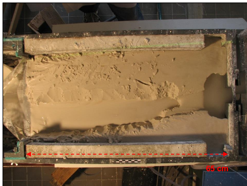
Fig. 3.2.2: Example of one of the images collected using the mounted time lapse camera. Flow is from right to left in this image. Also visible at the top edge of the flume, at the boundary between the paste and the wooden board is the green laser beam from the laser scanner.
