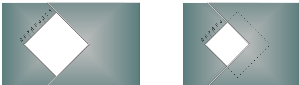
Figure 5.4: Schematic of the new orifice and damper settings. The numbers represent the damper setting used in Table 5.1.
