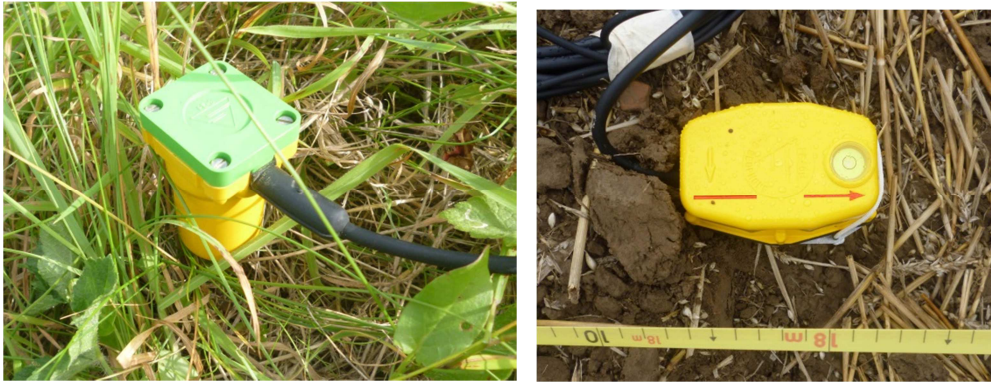
Figure 8.17 – In-situ placement of geophones
