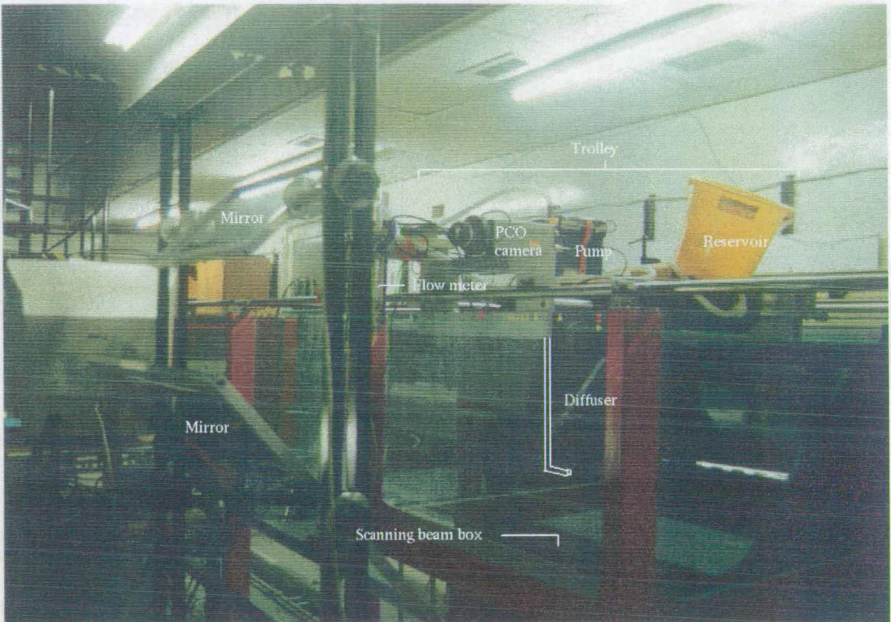
Figure 5.7: Experimental apparatus for round plume experiments
