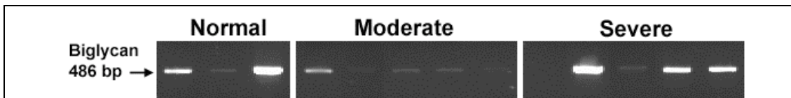
Figure 5.14. The gel electrophoresis picture shows the RT-PCR products for the biglycan gene (486 bp) after 31 cycles.
