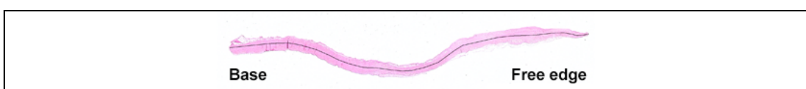
Figure 2.1. A schematic diagram shows how the central axis is plotted for leaflet length measurement.
