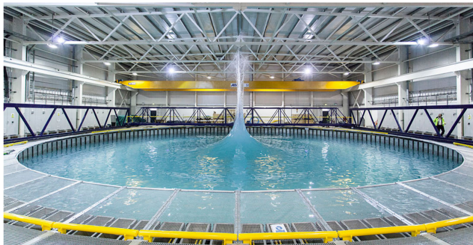
Figure 1.4: The FloWave concentric wave spike 'party trick'. Demonstrates accuracy of circular generating capability
