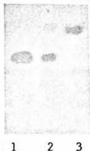
Figure 1. Thin layer alumina chromatography of 1, androstenediol (17 \alpha ); 2, the androstenediol (17 \alpha and \beta ) fraction from infant urine; and 3, androstenediol 17 \beta . The separation was achieved by 2 runs in System C, and colour development was by antimony trichloride. A part only, of the chromatography plate is shown.
