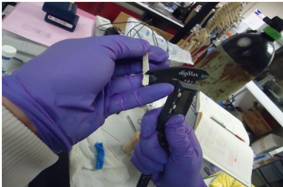
Figure 16- Electronic vernier callipers- Measuring the Thickness
