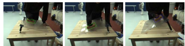
Fig. 10 Human wiping demonstrations on surfaces of varying tilt and rotations. The ASIMO stereo vision system was used to track the 3-D coordinates of the sponge ( coloured rectangles show the estimated position). Tilts of \pm 16^\circ and +27^\circ about the x -axis are shown
