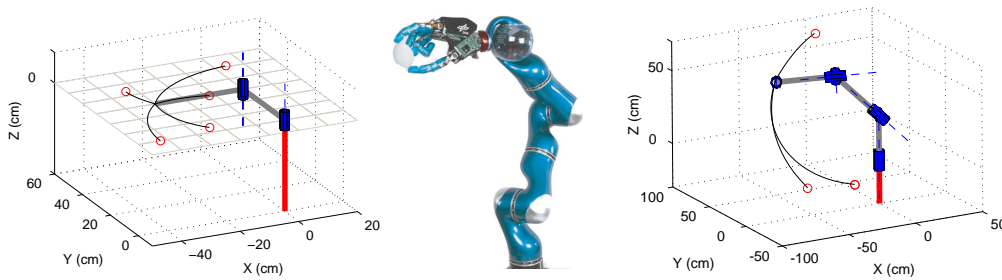
Figure 4.3: Two different joint-torque controlled manipulator models with selected targets (circles) and ILQG generated trajectories as benchmark data. All models are simulated using the Matlab Robotics Toolbox. Left: 2 DoF planar manipulator model; Middle: picture of the Kuka Light-Weight Robot arm (LWR); Right: Simulated 6 DoF LWR model (without hand).
