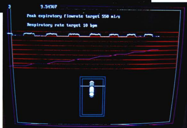
Figure A3.1. Ventilation targeting software screen displays. These prompt the user for ventilation target parameters such as expiratory flowrate and breaths per minute.
