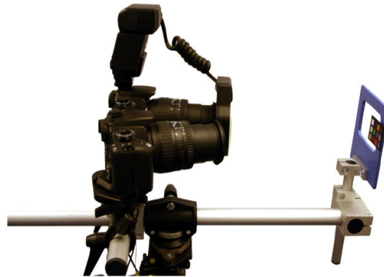
Figure 2.2: The dense stereo imaging system (DSIS)
