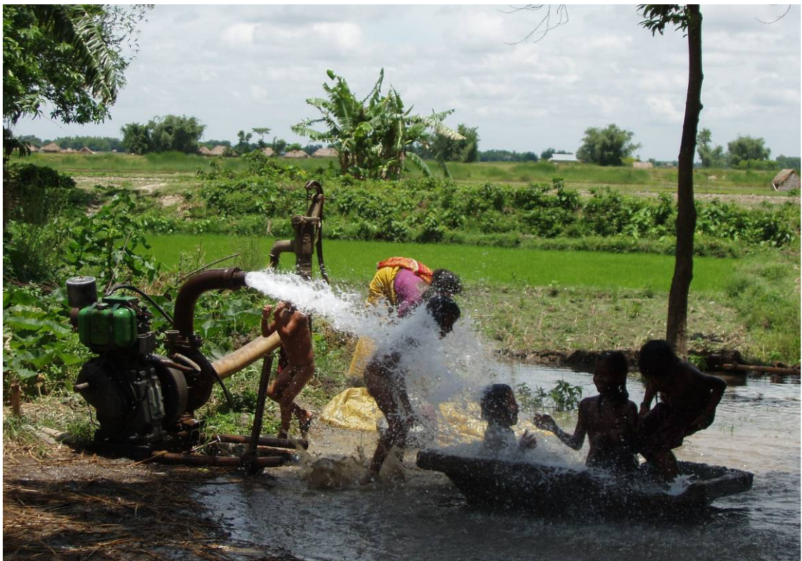
Figure 6-19: Shallow tube well drawing water from canal in Janghrahi: Although tubewell irrigation can significantly boost yields it is expensive
