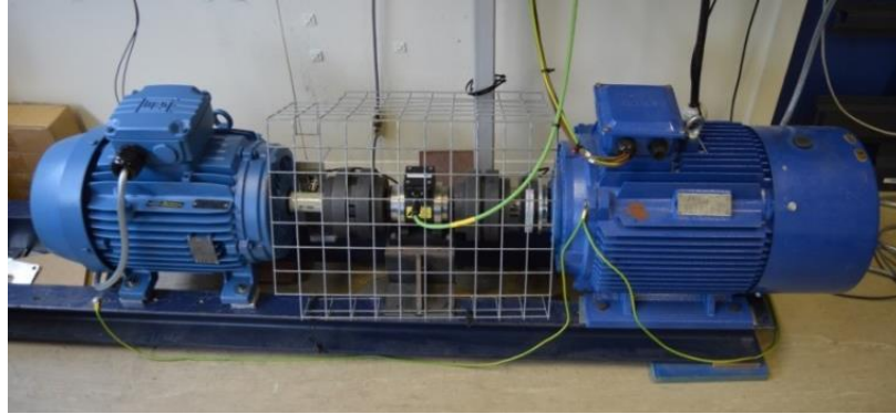
Figure 6.25: Coupling of the 22 kW induction motor (right) and the 11 kW induction generator (left)
