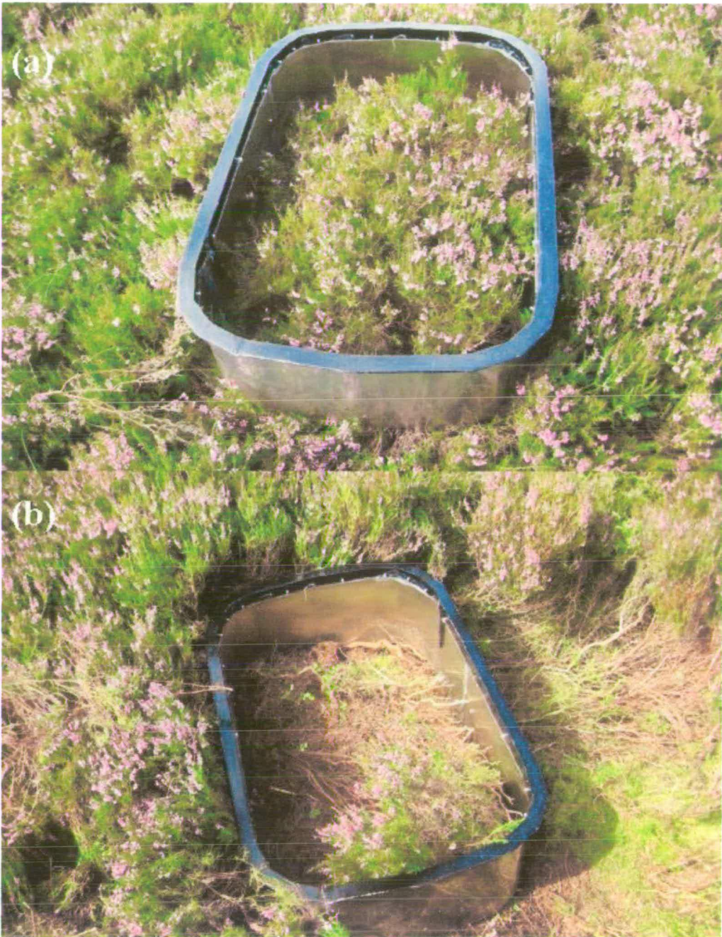
Figure 6.1: The effect of inserting chamber base into Calluna dominated bog. (a) before chamber insertion, (b) after chamber insertion.
