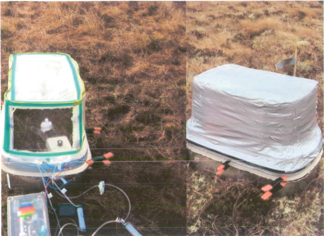
Figure 4.1: Light (left) and dark (right) chambers used for the measurement of \text{CO}_2 and \text{CH}_4 fluxes from blanket bog at Forsinard 2003-2005.
