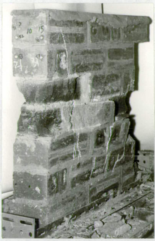
Figure 3.1 Failure of a 1:1/4:3 Mortar Wall - No WS9b
