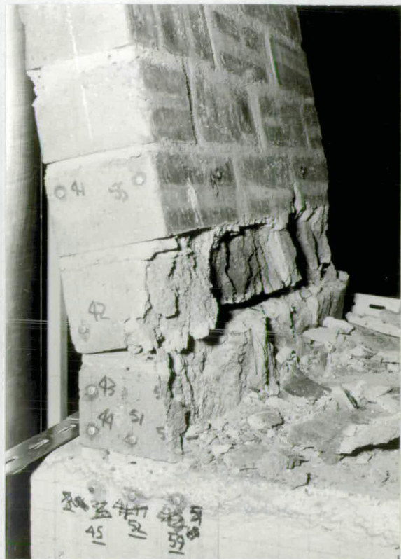
Figure 6.7 Wall Failure. 1:1:6 Mortar Wall Precompression 600 lbf/in 2
