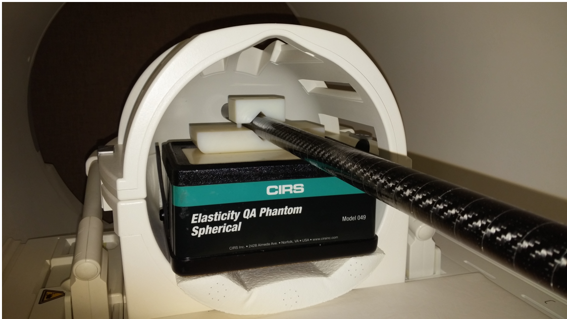
Figure 4.2: Setup for scanning the phantom. The carbon fibre rod transmitted waves from the loudspeaker.
