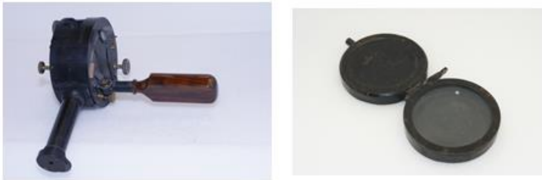
Fig 4.13: George's pattern double sextant and artificial horizon. 180
