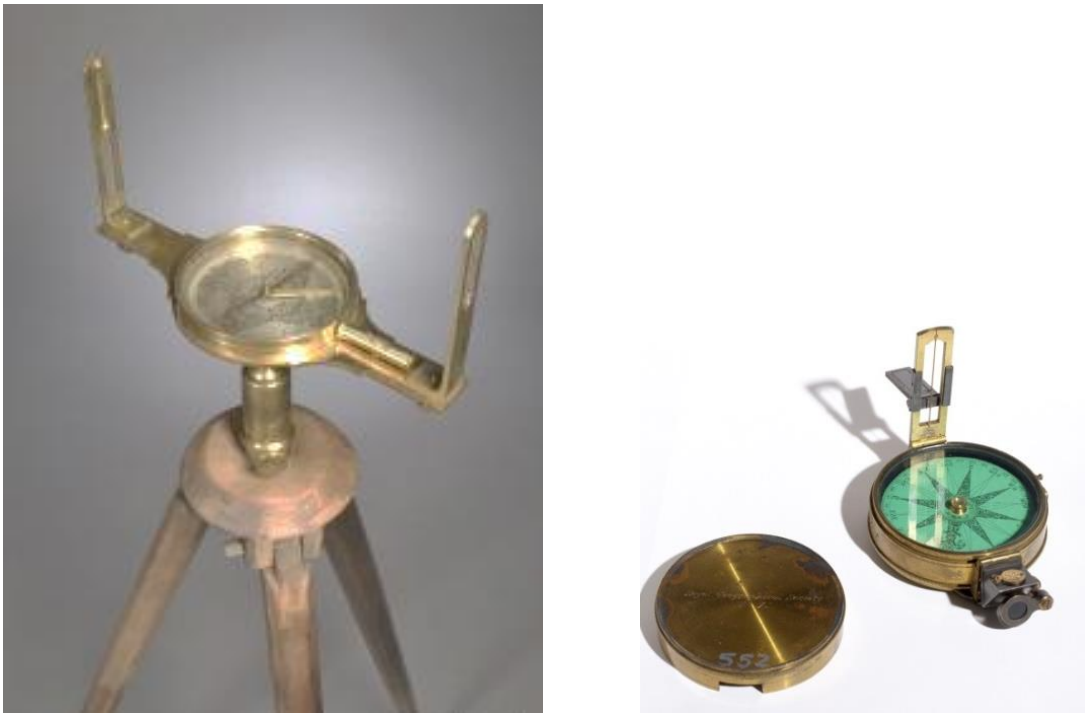
Fig 4.4: Changes in Compasses: Left, a surveyor's compass, right, prismatic compass used by Livingstone. 25
