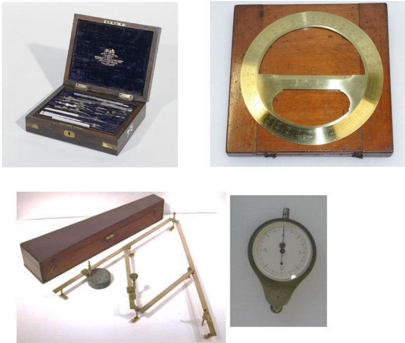
Fig 7.7: Drawing instruments. From top left clockwise: set used by Cameron in the mid nineteenth century, circular protractor by Cary 1892, passometer for map measuring by Cary 1894, and pantograph for enlarging and reducing drawings early to mid-nineteenth century. 76
