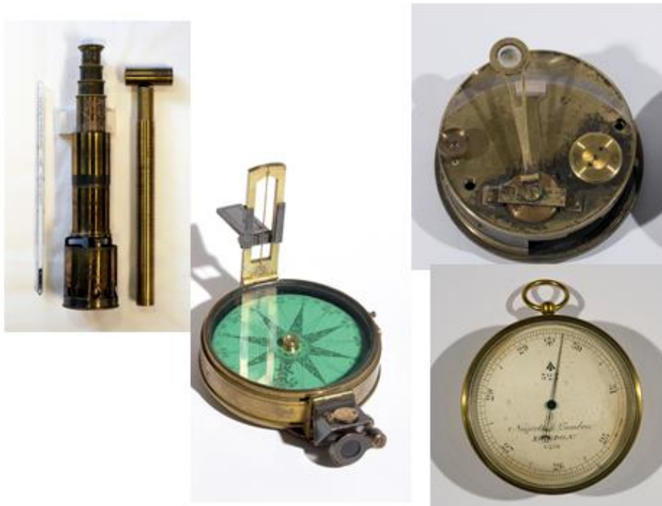
Fig 3.7: Instruments Commonly Used c.1860-c.1900: From left to right: hypsometer, prismatic compass, box sextant, and aneroid. 23
