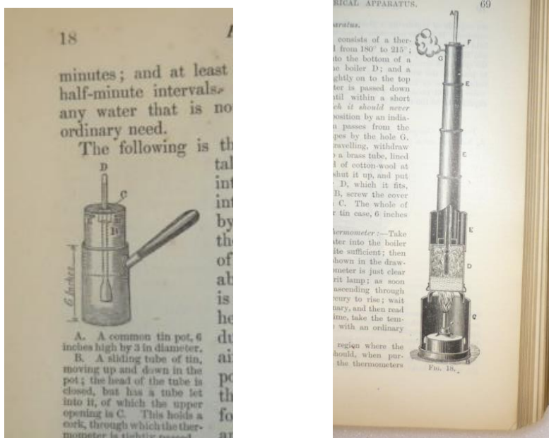
Fig 5.2 a, and b: Hypsometers from Hints (1865) and Hints (1906) respectively, demonstrating the more professional approach of the later editions.
