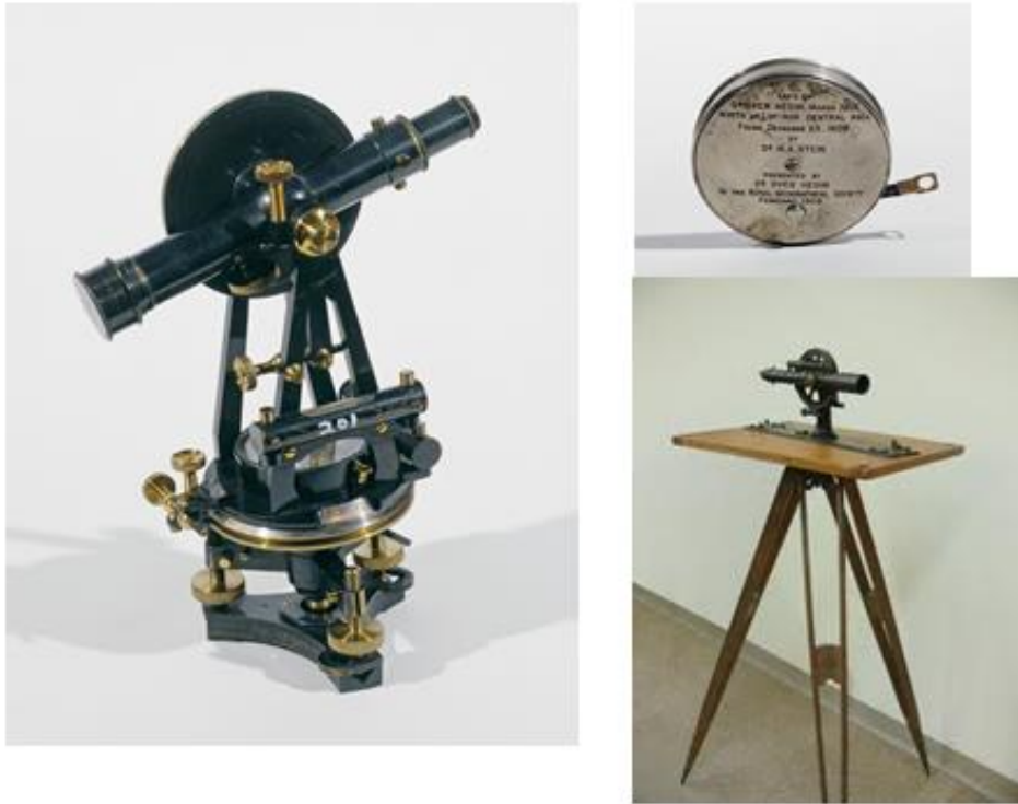
Fig 3.8: Instruments Commonly Used 1900-1930: From left to right: theodolite, tape measure, and plane table. 25
