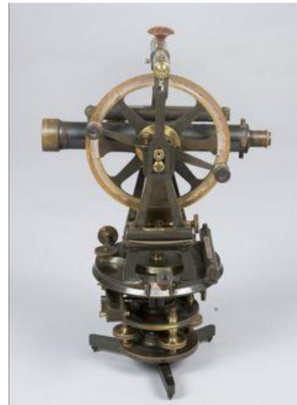
Fig 4.5: National Instruments: Left, astrolabe prism, and right, six inch transit theodolite by Troughton and Simms. 33
