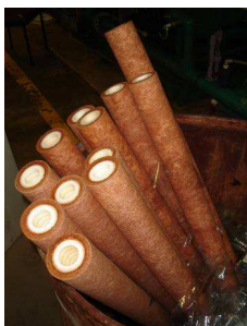
Figure 4 Filters for existing RO plants clogged by feed water iron content
