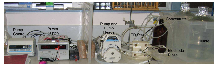
Figure 1 Electro dialysis System Layout with pump control, power supply, pump, ED stack, and three containers with electrode rinse, concentrate and diluate.
