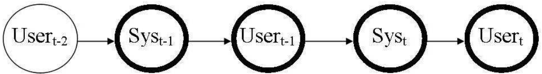
Figure 5.2: A representation of a portion of dialogue in which time is discrete, each unit of time contains one system-user exchange, and the arrows indicate the flow of the dialogue. A 4-gram simulation would output a new action for User_t depending on the actions at the previous turns that have bold circles.
